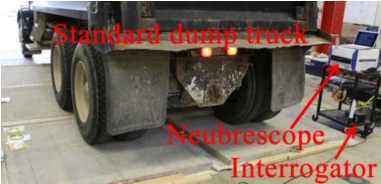
Fig. 5.4. Concrete panels under truck loads.
