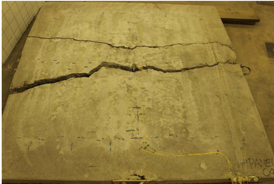
Fig. 6.13. Cracks in P4 after load frame test.
